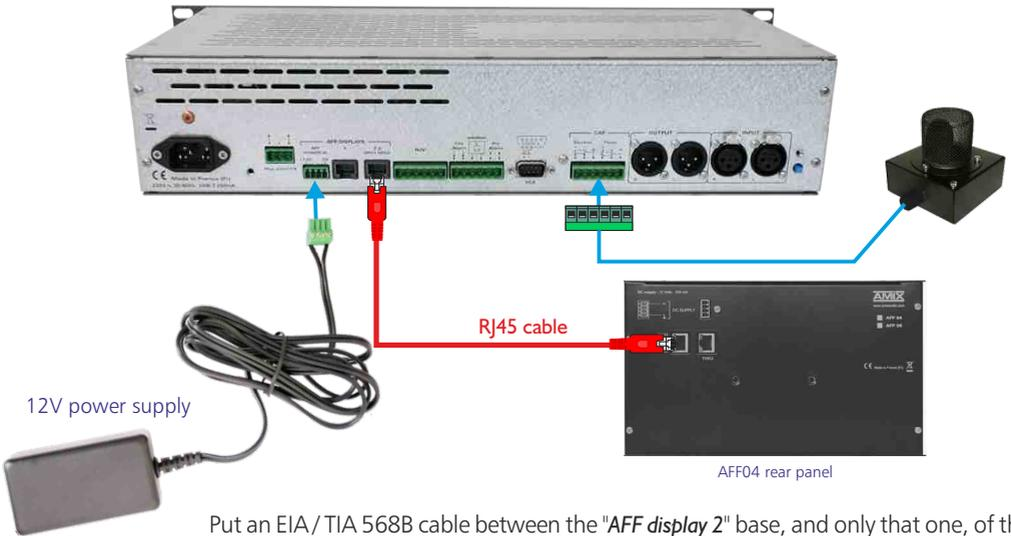
Put an EIA / TIA 568B cable between the "AFF display 2" base, and only that one, of the SNA and the RJ45 socket (GPO1 / GPO2) of the AFF04 (or AFF08) display. This cable carries both power and measurement modulation.
