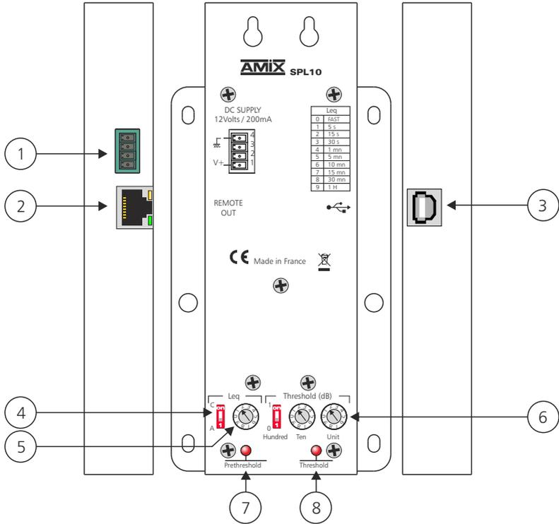
1: Power connector of the SPL10, only in case the SPL10 is used alone without the display.
